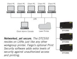
Windows®-based PC through its USB port. It can also be added to your network as easily as any workgroup printer. The optional Ethernet port and internal print server allow you to install and share the DTC550 anywhere you need it. And its print driver provides bi-directional status information, so you can monitor and manage the DTC550 just as you would any other networked printer.
